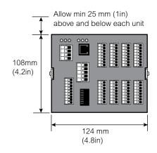
Allow a minimum of 25mm (1in) for terminals and cables in front of the unit.
