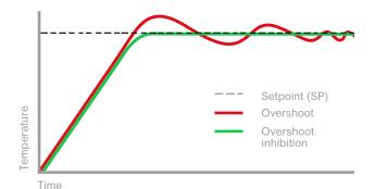
By automatically reducing power demand near the setpoint the Eurotherm cut back feature significantly minimizes overshoot which reduces waste and optimizes energy usage. This lowers the risk of parts not reaching operating temperature or overheating.
