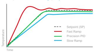
Ramp rate controls the rate of change to setpoint, keeping the material within specified temperature limits, minimizing damage and distortion in the final product. A holdback "Guaranteed Soak" function enables material to reach the required temperature before the process advances.
