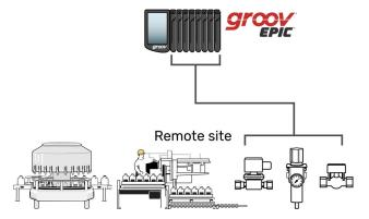
If existing controls are in place already, they can be connected to a segmented network interface on the EPIC, which can use OPC UA drivers to pull the data in.
