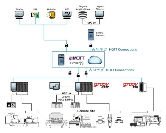
This approach is open, flexible, and powerful. With MQTT/Sparkplug B as the backbone of the network, up-front licensing costs are significantly limited, and there is no reason to be locked into a particular network configuration.
