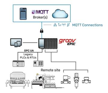
Now, applications can be plugged into the infrastructure. A gateway application, like Ignition Gateway with Cirrus Link's MQTT Engine, can subscribe to the entire system's tags and make all that data available to other applications, including back into OPC, if needed.
