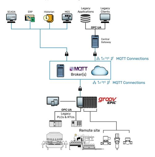
With this foundation, the system can scale up with additional edge devices or additional brokers to build out a highly resilient, high-performance data exchange and command-and-control system that's completely secure.
